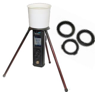
Set of accessories for 137 Cs activity and αβ flux density measurement
